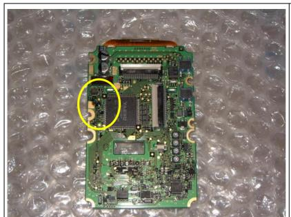
Remove cables an turn the board like this.
