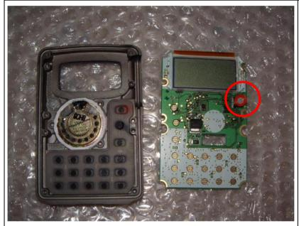
Now we will give the internal electret microphone a little more brightness and clearance of its sound.
