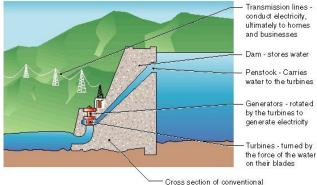
hydropower facility that uses an impoundment dam
