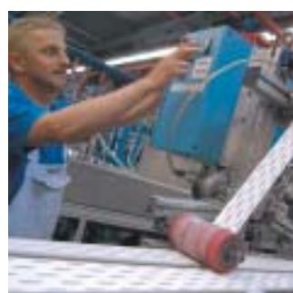
*Extrusion is a technique used to manufacture high-grade plastic elements for Tehalit systems.*
