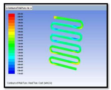
Fig 24: HEAT TRANSFER COEFFICIENT
